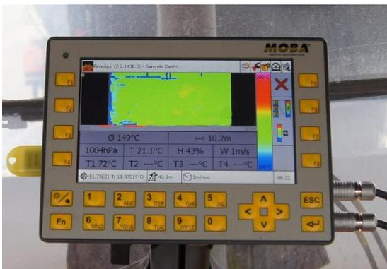
*The temperature profile is displayed on the computer and at the same time recorded for later analysis*
